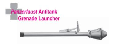
**Operation** Grenade launcher, percussion fired
